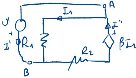
$$\left. \begin{aligned} U' &= I' R_1 - I'' R_1 \\ I'' &= I_1 + I' \rightarrow I_1 = I'' - I' \end{aligned} \right\} U' = -I_1 R_1 \quad *$$
