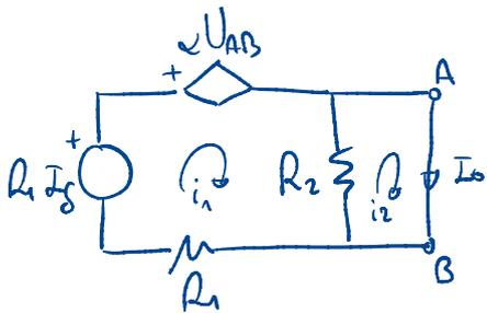
$$i_1 \rightarrow -\alpha U_{AB} + R_1 I_S = i_1 (R_1 + R_2) - i_2 R_2 \rightarrow$$
