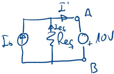
$$\left. \begin{aligned} I_0 &= I' - I_{eq} \rightarrow I' = I_0 + I_{eq} \\ I_{eq} &= \frac{10}{2} = 5 \text{ A} \end{aligned} \right\} I' = 20 + 5 = 25 \text{ A}$$
