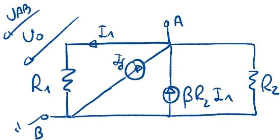
$$I_S + \beta R_2 I_1 = U_{AB} \left( \frac{1}{R_1} + \frac{1}{R_2} \right) \rightarrow$$
