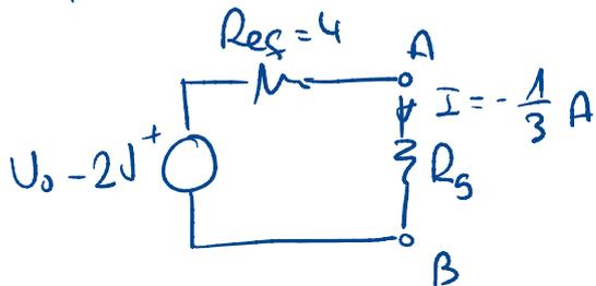
$$U_0 = I (R_{eq} + R_S) \rightarrow R_S = \frac{U_0}{I} - R_{eq} \rightarrow$$
