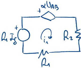
$$i_1 R_1 I_S - \alpha U_{AB} = i_1 (R_1 + R_2) \rightarrow R_1 I_S = i_1 (R_1 + R_2 (1 + \alpha))$$
