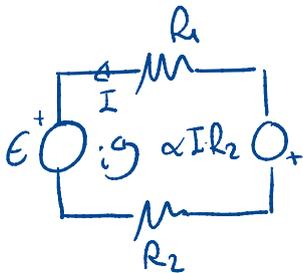
$$\text{P)} -E - \alpha I R_2 = i (R_1 + R_2) \xrightarrow{i=I} -E = I (R_1 + R_2 (1 + \alpha)) \rightarrow$$
