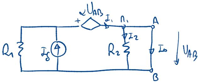
$$U_{AB} = I_2 R_2 = (I_1 - I_0) R_2$$
