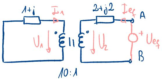
$$\left. \begin{aligned} 0 &= (1+j)I_1 + U_1 \Rightarrow U_1 = -(1+j)I_1 \\ U_1 &= 10U_2 \end{aligned} \right\} \left. \begin{aligned} 10U_2 &= -(1+j)I_1 \Rightarrow U_2 = \frac{-(1+j)I_1}{10} \end{aligned} \right\}$$
