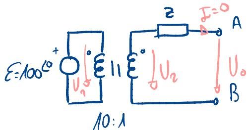
$$\left. \begin{array}{l} E = U_1 \\ U_1 = 10U_2 \\ U_2 = U_0 \end{array} \right\} U_0 = \frac{E}{10} = 10 \angle 0^\circ$$
