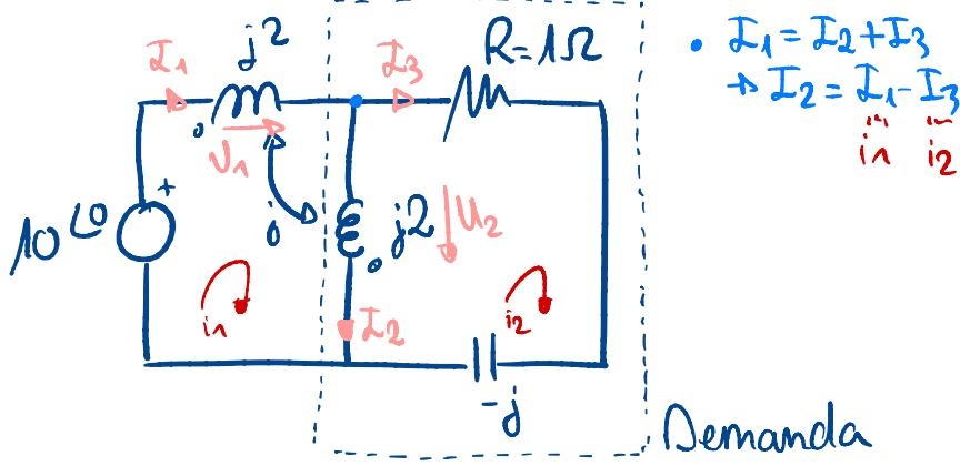
$$\begin{aligned} I_1 &= I_2 + I_3 \\ \rightarrow I_2 &= I_1 - I_3 \end{aligned}$$
