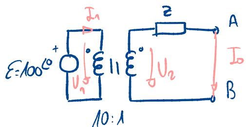
$$\left. \begin{array}{l} E = U_1 \\ U_1 = 10U_2 \\ U_2 = E/Z \end{array} \right\} E = 10I_o Z \rightarrow I_o = \frac{E}{10Z} = \frac{100^{\circ}}{10 \frac{20\Omega(1+j)}{100}} = \frac{500(1-j)}{20\Omega}$$
