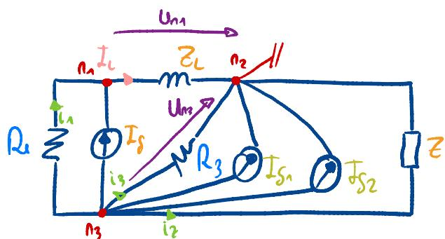
$$I_{S1} = \frac{E_s}{R_3} = \frac{60 \angle 90^\circ}{3} = 20 \angle 90^\circ$$
