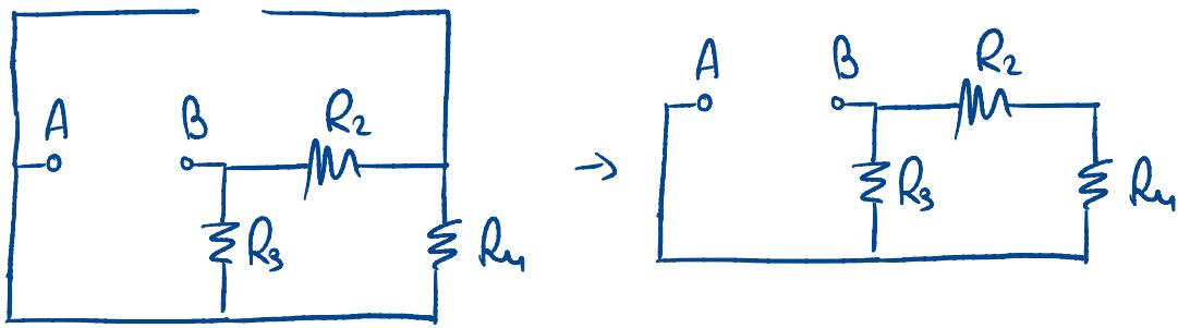
$$R_{eq} = \frac{1}{\frac{1}{R_3} + \frac{1}{R_2 + R_L}} = \frac{1}{\frac{R_2 + R_L + R_3}{R_3(R_2 + R_L)}} = \frac{R_3(R_2 + R_L)}{R_2 + R_L + R_3}$$
