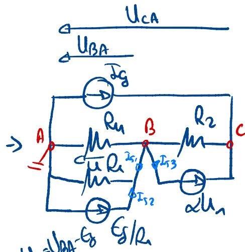
$$B: \frac{E_s}{R_1} - \alpha U_1 = U_{BA} \left( \frac{1}{R_1} + \frac{1}{R_2} + \frac{1}{R_3} \right) - U_{CA} \frac{1}{R_2} \xrightarrow{U_n = U_{BA} - E_s / R_1} E_s \left( \frac{1}{R_1} + \alpha \right) = U_{BA} \left( \alpha + \frac{1}{R_1} + \frac{1}{R_2} + \frac{1}{R_3} \right) - U_{CA} \frac{1}{R_2}$$
