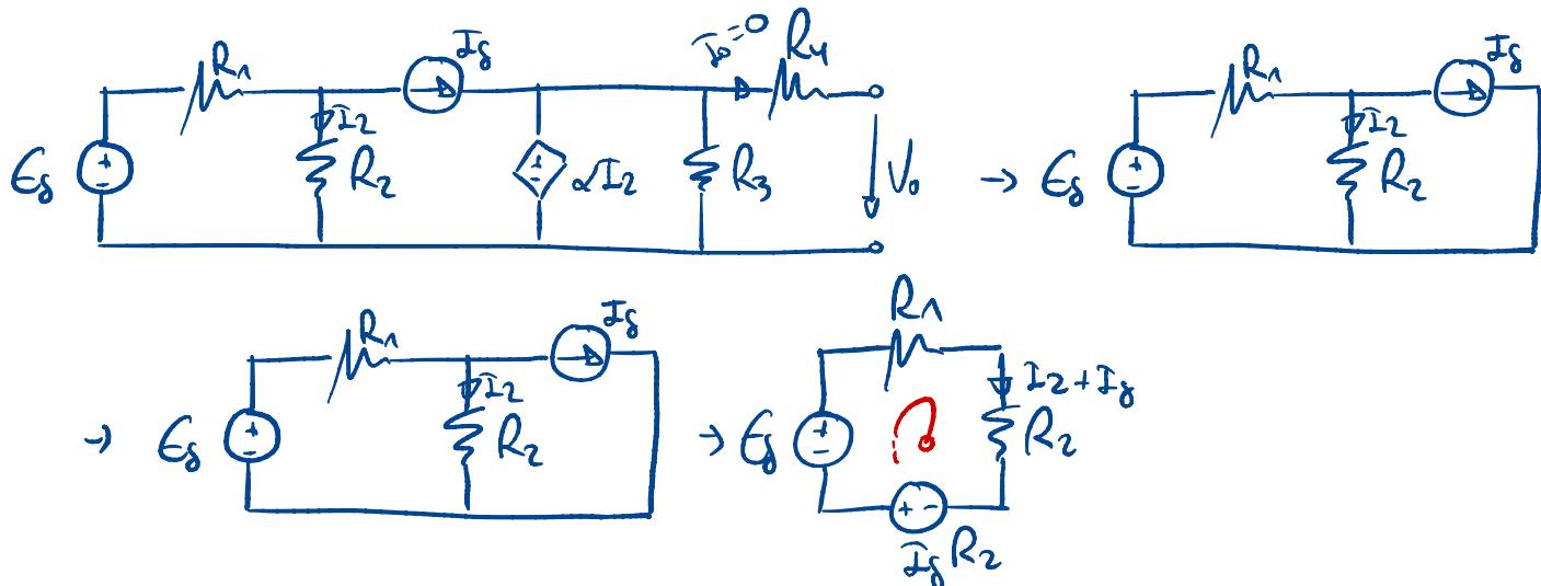
$$\text{?} \quad E_8 + I_8 R_2 = i(R_1 + R_2) \rightarrow i = \frac{E_8 + I_8 R_2}{R_1 + R_2}$$
