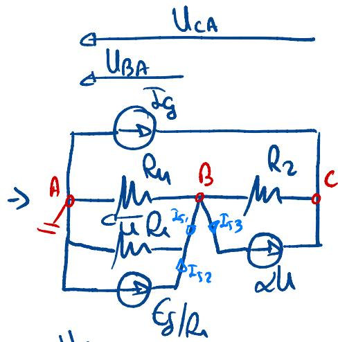
$$B. \frac{E_S}{R_1} - \alpha U = U_{BA} \left( \frac{1}{R_1} + \frac{1}{R_2} + \frac{1}{R_3} \right) - U_{CA} \frac{1}{R_2} \xrightarrow{U=U_{BA}} \frac{E_S}{R_1} = U_{BA} \left( \alpha + \frac{1}{R_1} + \frac{1}{R_2} + \frac{1}{R_3} \right) - U_{CA} \frac{1}{R_2}$$
