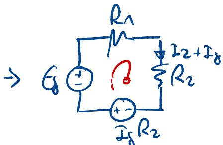
$$\text{? } E_s + I_s R_2 = i(R_1 + R_2) \rightarrow i = \frac{E_s + I_s R_2}{R_1 + R_2}$$
