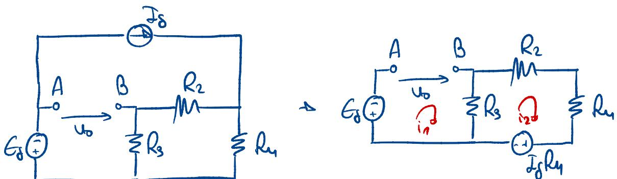
$$i_1 - E_s = i_1 R_3 - i_2 R_3 \xrightarrow{i_1=0} -E_s = -i_2 R_3$$
