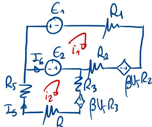
$$i_1 \rightarrow -E_1 - \beta U_S R_2 - E_2 = i_1 (R_1 + R_2) \xrightarrow{U_S = i_2 R_3} -E_1 - E_2 = i_1 (R_1 + R_2) + i_2 \beta R_2 R_3$$
